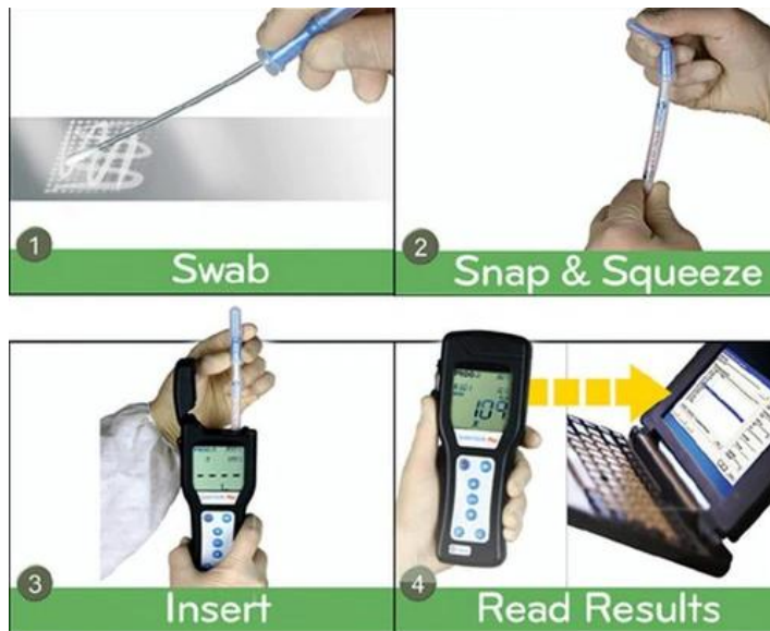
Fig. 15.3. Work with the luminometer (Hygenia SystemSURE Plus ATP Monitor ( qasupplies.com ))
