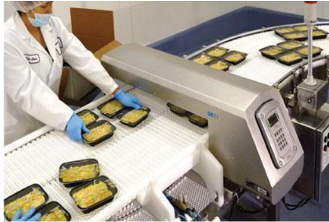
Fig.18.2. Critical control point - detection of foreign bodies
